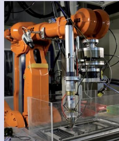
Robotic arm and laser head during the process of surface coating.
