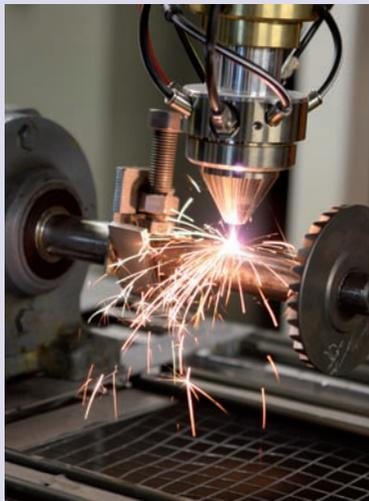
Laser surface coating of a tractor axis.
